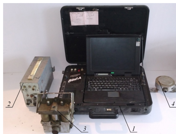
3: General view of the electronic measuring system designed to measure fuel consumption and travel speed
