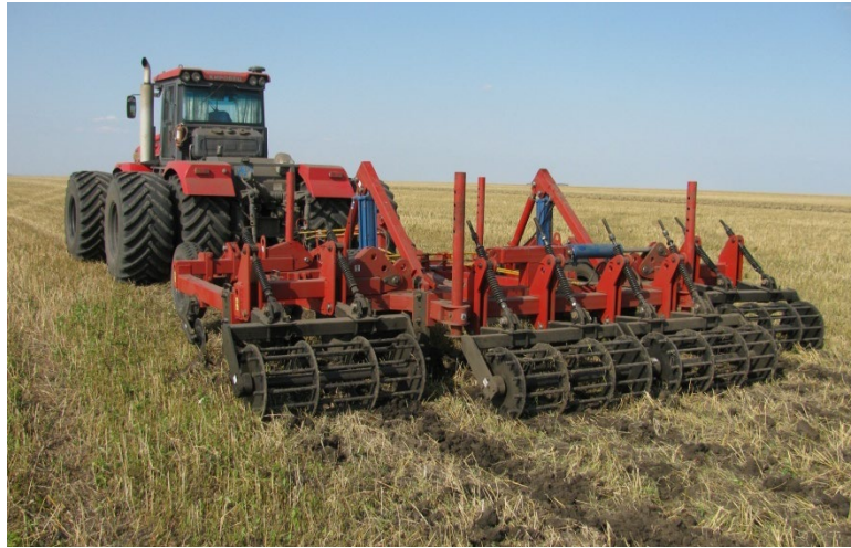
7: Experimental model of the tillage implement aggregated with the tractor «Kirovets» K-744P2
