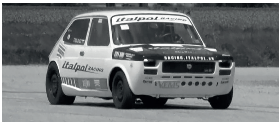
1: Modified race car FIAT 127 equipped with motor Lancia 2.0 16V, 310 kW Source: own
