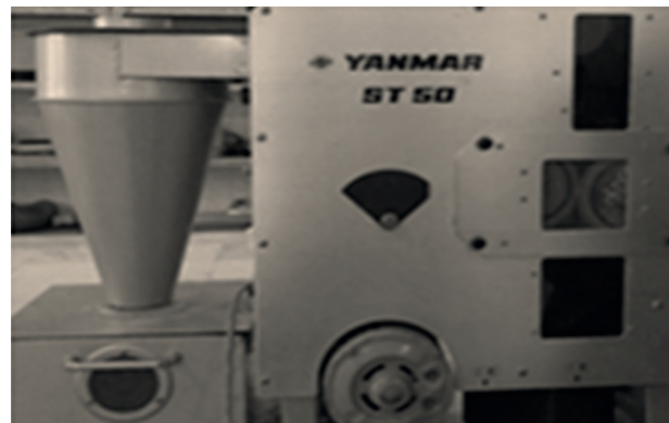
1: The machine (Yanmar type) which is used for hulling rice
