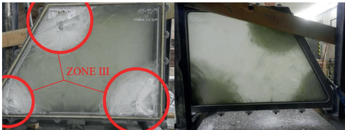
6: Degraded side glass after shooting tests using projectile 7.62 × 54R B32 API at the temperature of -32 °C
