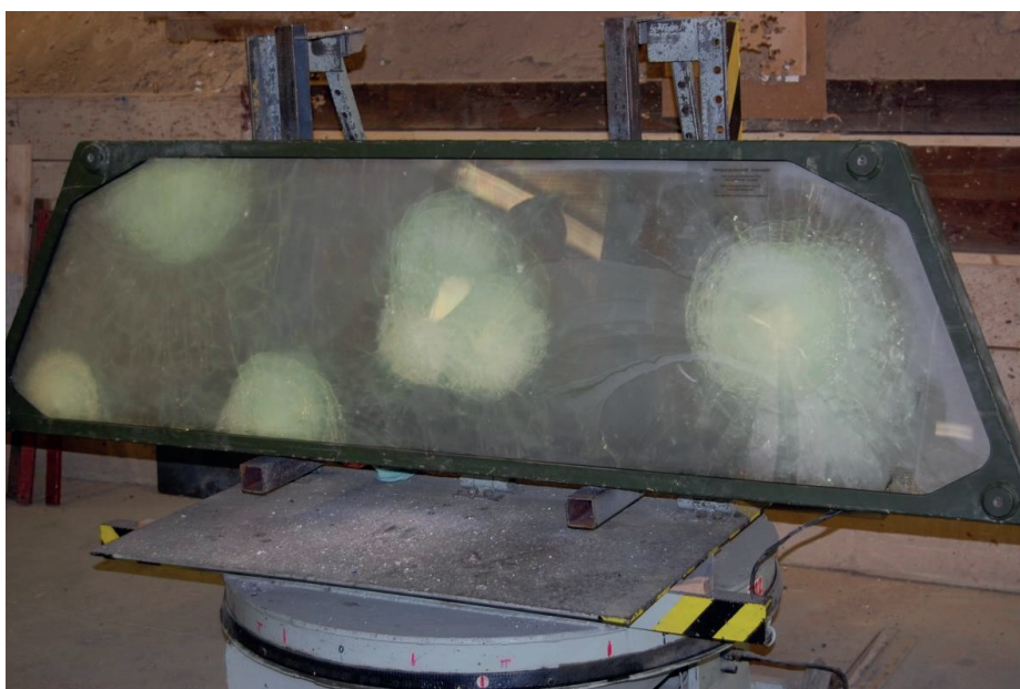
4: Glass after shooting tests using projectile 7.62 \times 54R B32 API and 7.62 \times 39 API BZ inner side
