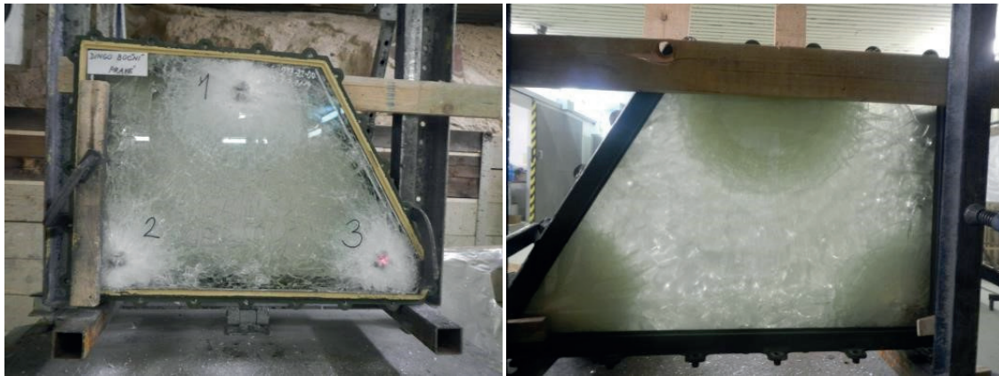
5: Glass after shooting tests using projectile 7.62 × 54R B32 API
