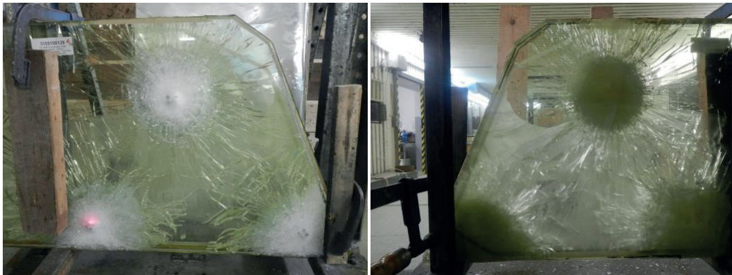
2: Glass after shooting tests using projectile 7.62 × 54R B32 API
