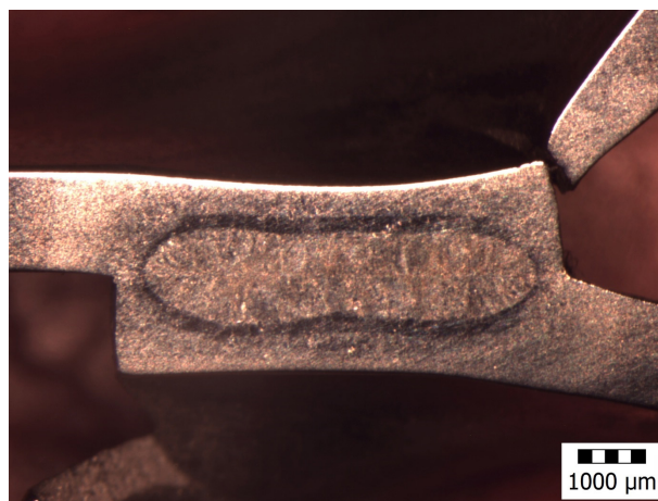
2: Macrostructure of spot weld, sheet thickness 1.5 + 1.5 mm, t = 2.0 s
