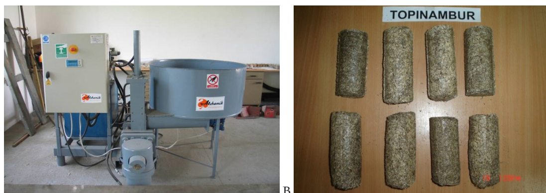
5: A – Alchemik press machine and B – briquettes from Miscanthus sinensis
