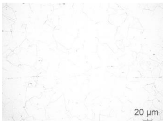
16: Sample 1-J5 400:1 Base material \text{HNO}_3 , \text{HCl}
