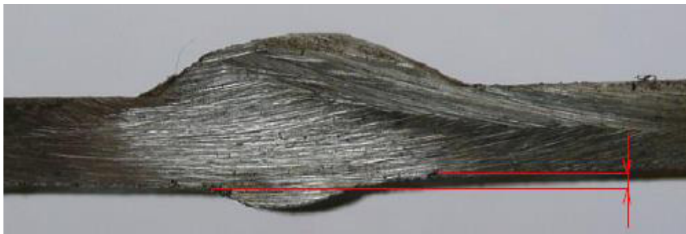
4: Detail Off-set root of weld
