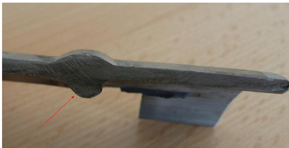
2: Internal protrusion in root of weld
