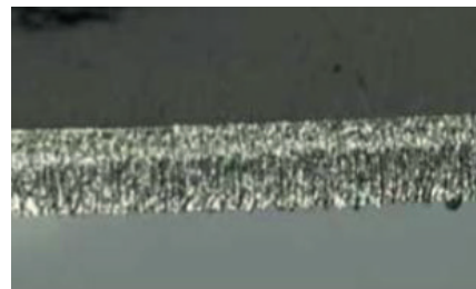
10: Cutting with beam pattern (2.4 m/min). (Hoult, 2006)
