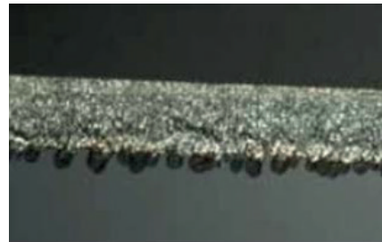
9: Cutting with one laser beam (2.1 m/min). (Hoult, 2006)
