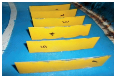
6: The vanes with six types of curvatures
