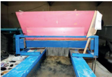
4: Sediment injection machine
