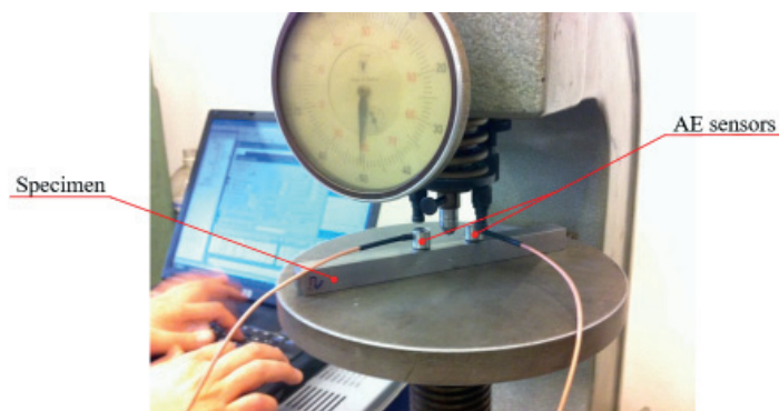
1: Location of AE sensors on a steel specimen during measuring Rockwell hardness Source: author
