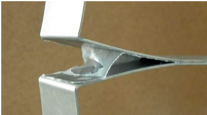
5: Initiation of failure area – adhesive type of failure of adhesive bond (treatment D)
