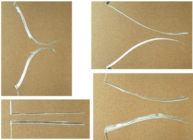
6: Different deformations of test specimens depending on treatment of adhesive bonded surface
