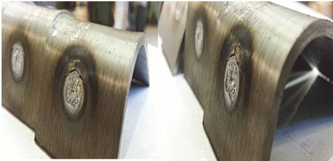
11: Brittle breach of steel weld ČSN 19 312
