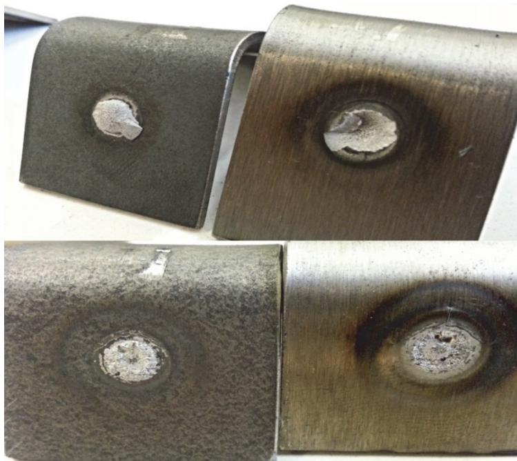
12: Breach at combined sample; centre in steel 11373 (left), brittle breach at non-welding 19312 (right)
