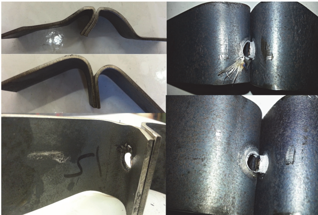
10: Plastic deformation "gape opening" of steel weld 11373
