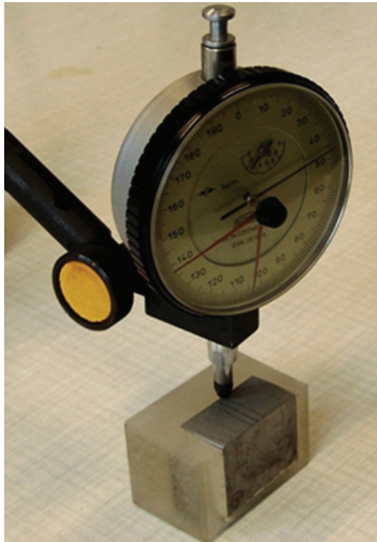
5: Flatness measuring device SOMET
