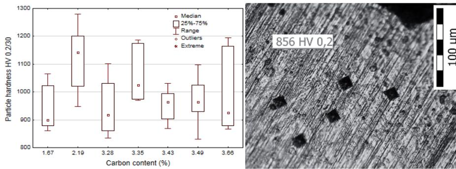
5: Particle hardness (left) and tested surface (right)
