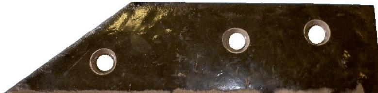
9: Prototype with renovated surface from composite with particles from machining process
