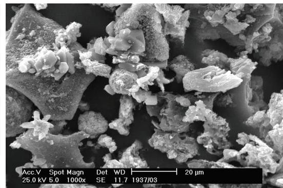
3: Configuration of hard residues – bed and filter ash
