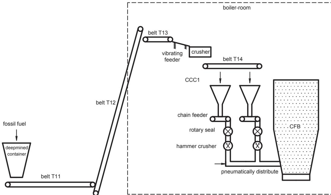
1: The scheme of the distribution and the fuel ratio to the boiler
