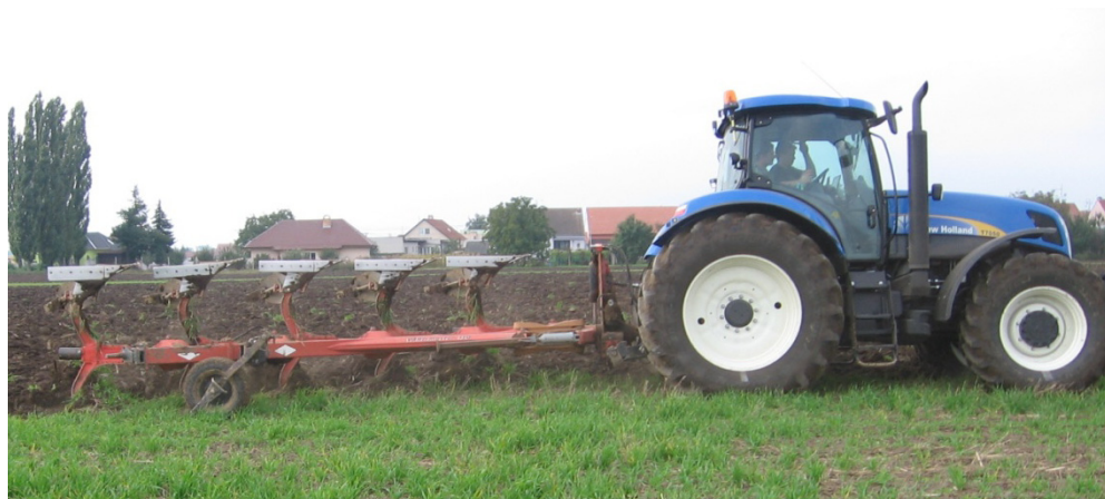
1: The combination of the tractor NewHolland T7050 in aggregation with the plough Kuhn Huard Variomaster 150
