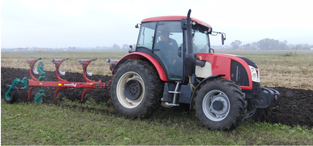
2: The combination of the tractor Zetor Proxima Plus 115 in aggregation with the plough Kverneland 150 B
