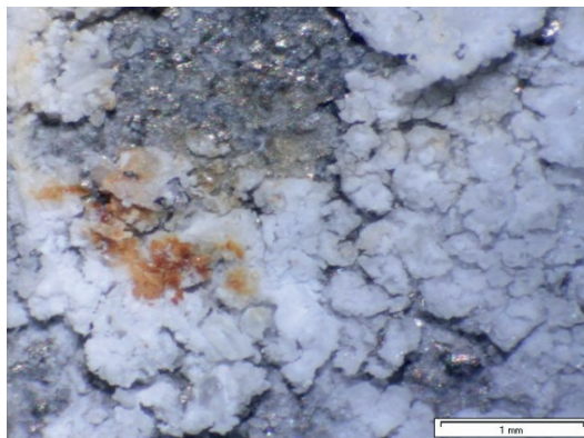
4: Blistering and point corrosion of duplex (left) and zinc coating (right)
