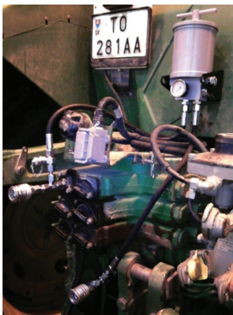
2: Additional filtration system and its mounted on big tractors
