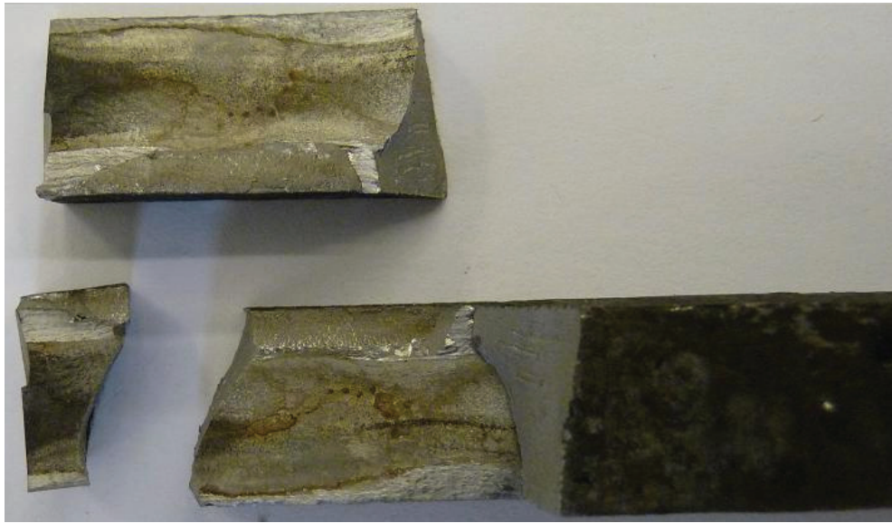
14: Delaminating at the weld (water/150°C, the force perpendicular to the plane of layers) (author)
