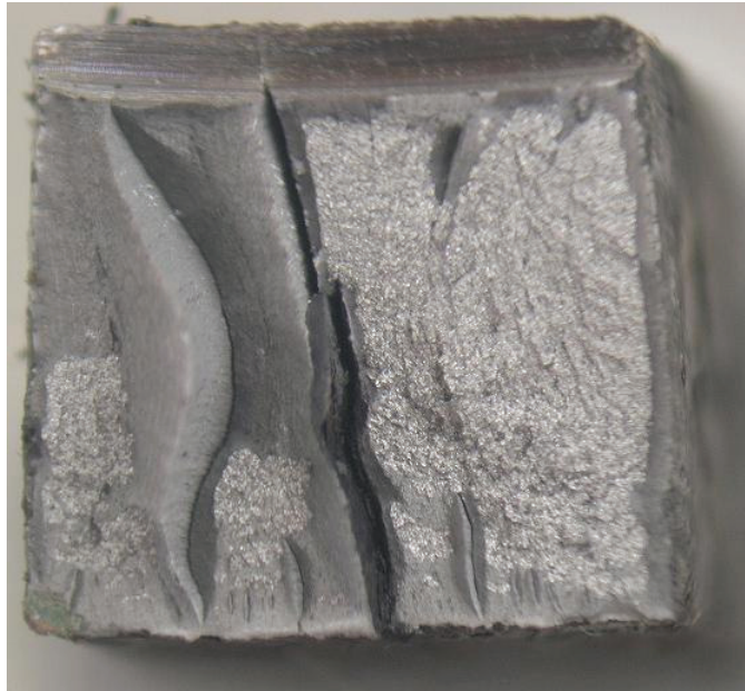
16: Transgranular and intergranular impact fracture on fission in line damask layers (oil / 350 °C) (author)
