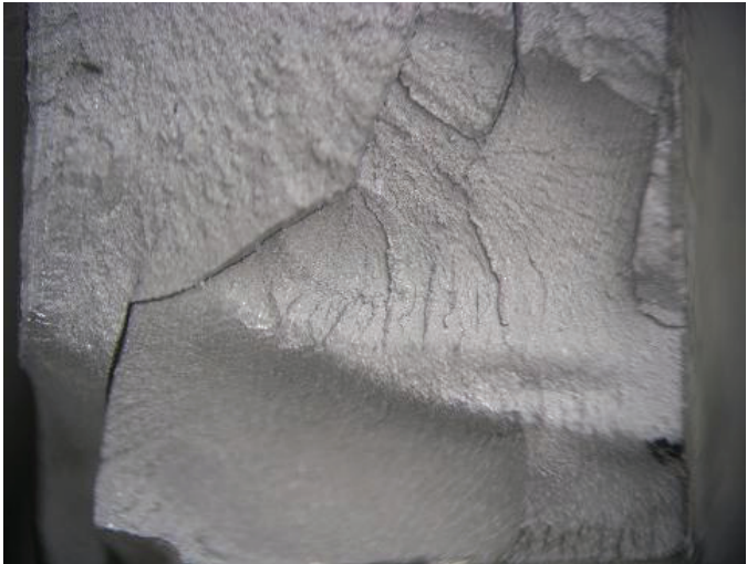
13: Fracture interconnection of layers (hardened to water/150 ° C, the direction of the layers line) (author)
