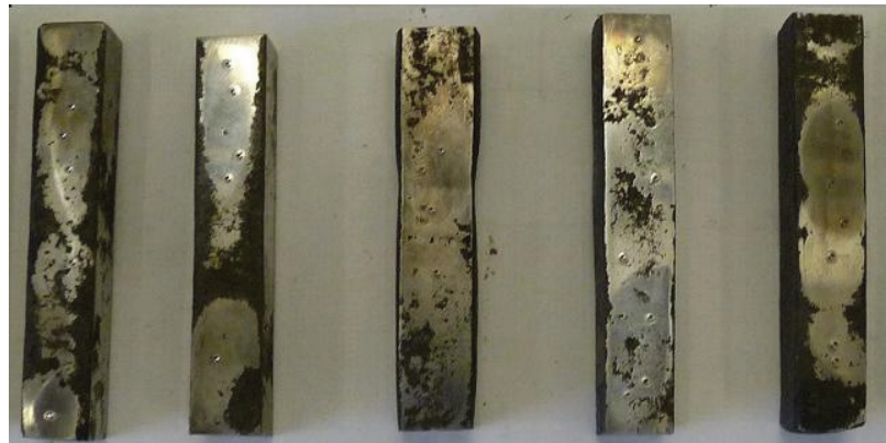
6: A set of ground samples for Charpy test after test hardness in natural untreated state, (author)
