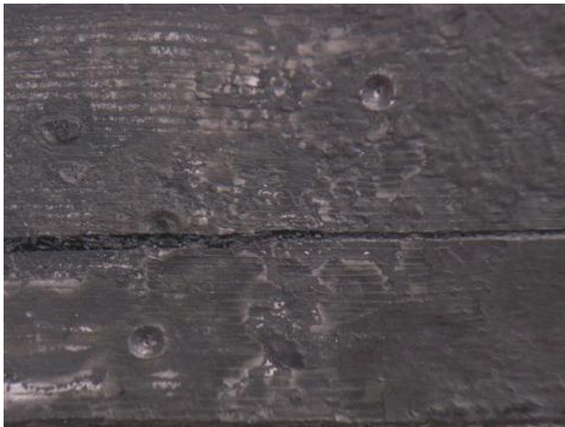
12: Rupture of weld between the layers after unsuccessful impact test (author)
