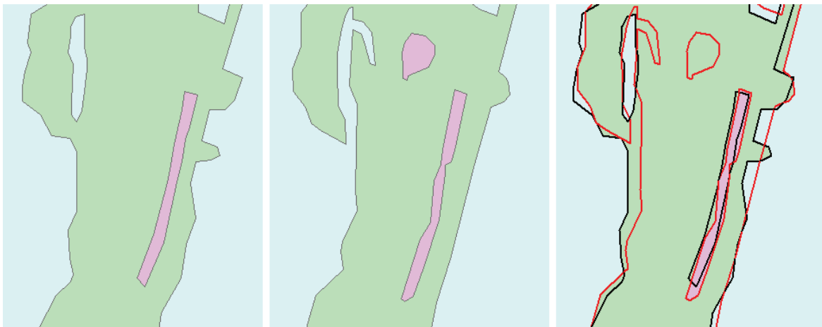
1: An example of correct layer integration. 1990 layer (left), 2006 layer (middle) and corrected 1990 layer (right) with highlighted lines originating both from the older (black) and the newer (red) layer.
