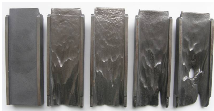
3: Erosive wear of an air-blast blade
