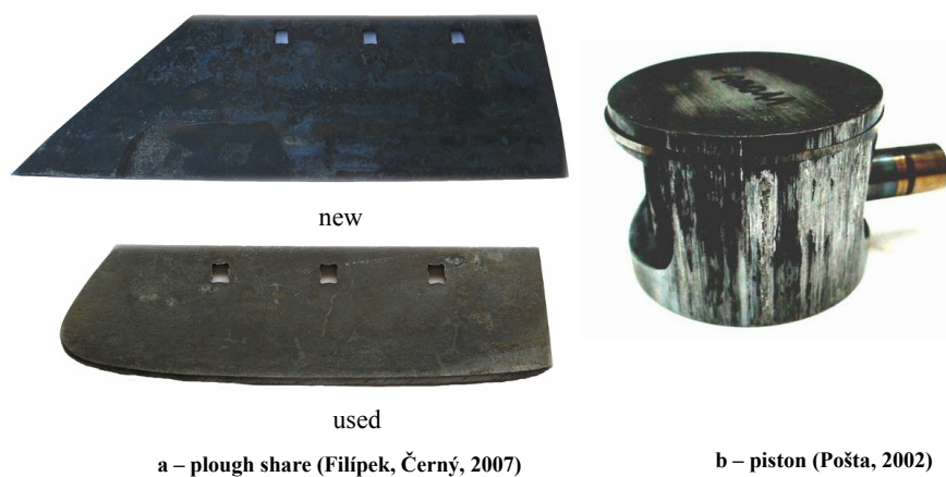
2: Examples of abrasive wear
