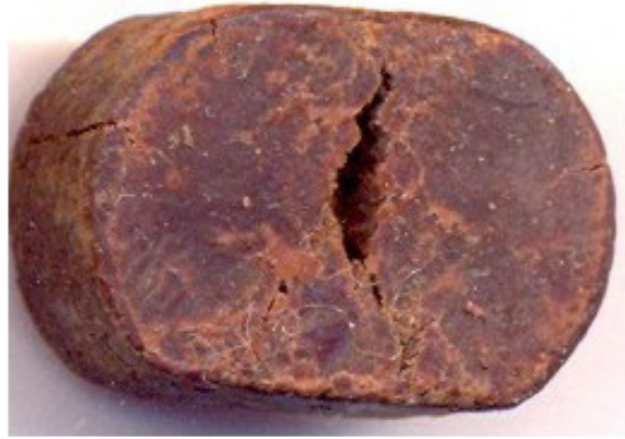
4: Specimen of the chocolate after the brasilian test. Crosshead velocity: 10 mm/min.
